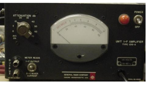
These meters provide a 30 MHz IF amplifier with up to several MHz of bandwidth which makes it easy to measure sun and moon noise – they can be easily retuned for 28 MHz
